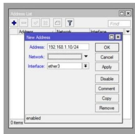
Gambar 13. Address IP Address
