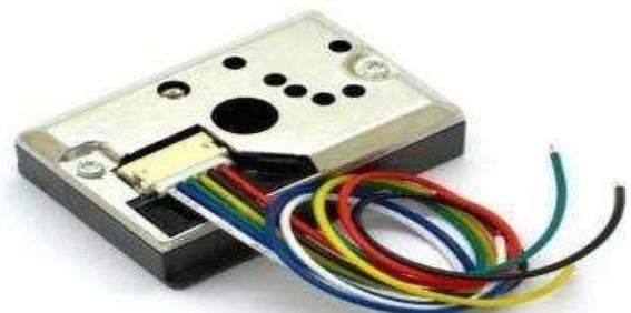
Gambar 5. Sensor debu GP2Y1010AU0F
