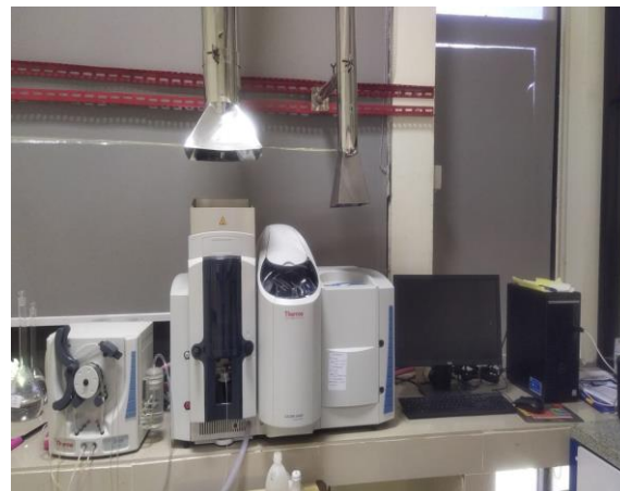
Gambar 2. Alat Atomic Absorption Spectrometry (AAS) Type Thermo Scientific ICE 3000 SERIES
