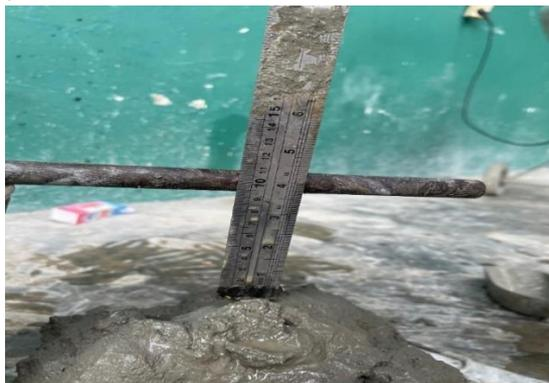
Gambar4. Slump Test
